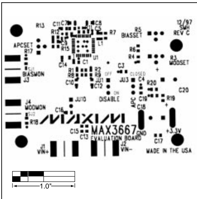
Figure 3. MAX3667 EV Kit Component Placement Guide
